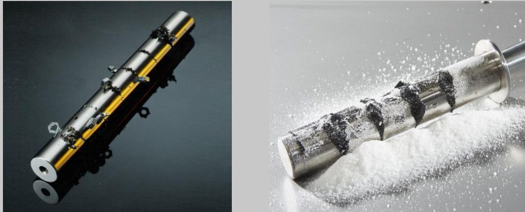
Magnetic bars used in magnetic separation systems. Particles collect on the tube near the pole plates because the Force Index is highest there.
